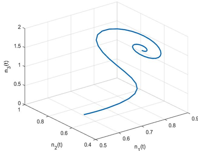
**Fig. 6.** The system is asymptotically stable at the point E (0.8415, 0.676, and 1.322).
