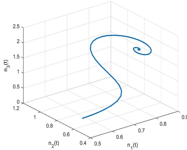
Fig. 4. The system is asymptotically stable at E (0.8327, 0.6967, and 1.777).
