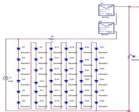
Fig.(7): PV arrays wired in series
