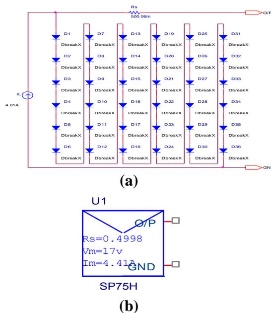
**Fig(1): (a)The electrical circuit of the PV model**
