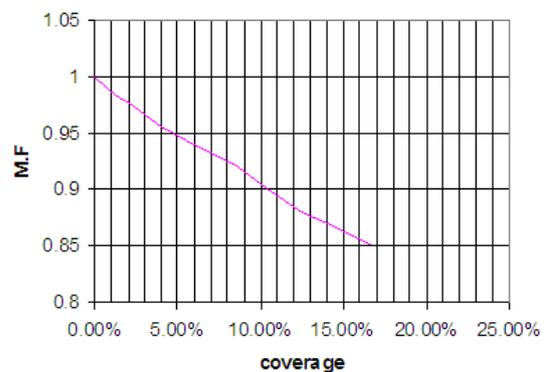
**Fig.(4): Mismatch factor for different amount cell shading**
