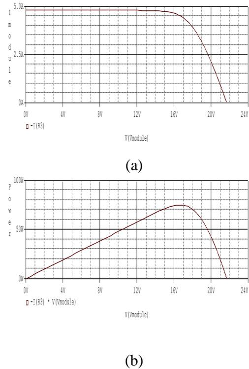
**Fig(2): (a) The I-V curves of the PSPICE PV module model**
