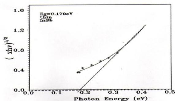
**Fig. (10) the value of optical energy gap for InSb thin film specimen**
