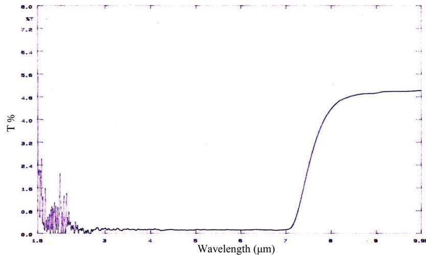
**Fig.(6) Transmission as a function of wavelength for InSb crystal**
