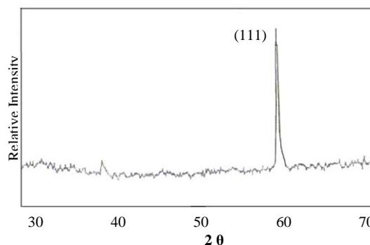
**Fig.(4) the X-Ray Diffraction patterns of InSb crystal prepared**
