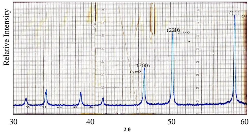
**Fig.(5) :the XRD patterns of deposited InSb thin films.**
