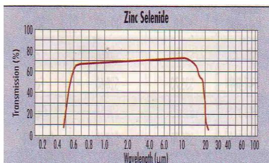
**Fig.(3) :The transmittance spectrum of ZnSe substrate**
