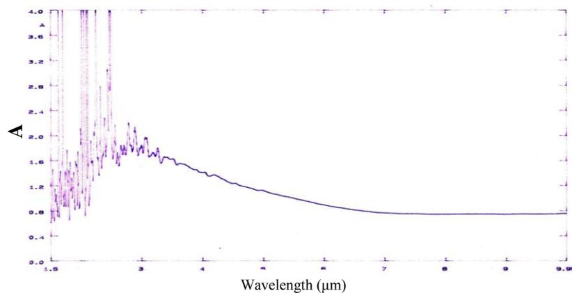
**Fig.(9) Absorption as a function of wavelength for InSb thin film**
