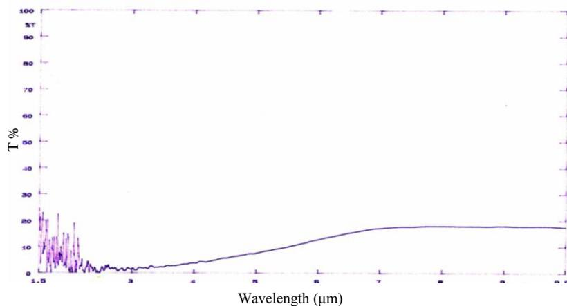
**Fig.(8) Transmission as a function of wavelength for InSb thin film**
