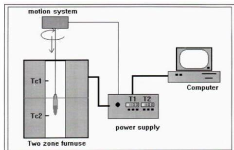
**Fig.(1) crystal growth system (vertical)[10]**
