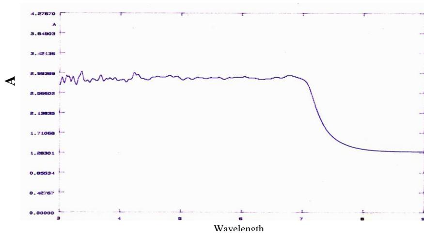
**Fig.(7) Absorption as a function of wavelength for InSb crystal**
