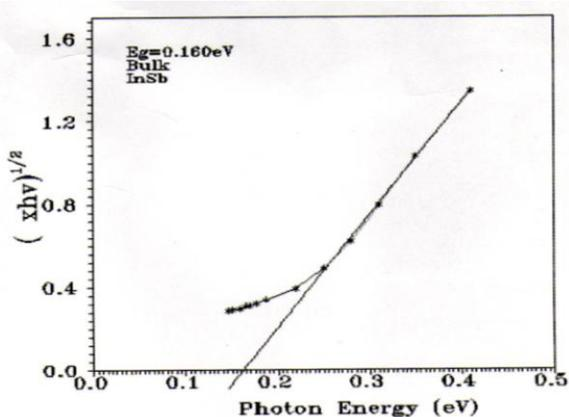
**Fig.(11) the value of optical energy gap for InSb single crystal specimen**
