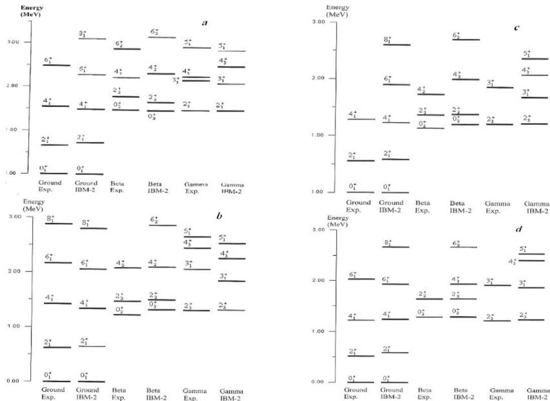
**Fig. (2): A comparison between the experimental low-lying positive parity states and those obtained by IBM-2a) <sup>110</sup>Cd [2,10,11], b) <sup>112</sup>Cd [4, 10, 11], c) <sup>114</sup>Cd [5,10,12], d) <sup>116</sup>Cd [10,13].**
