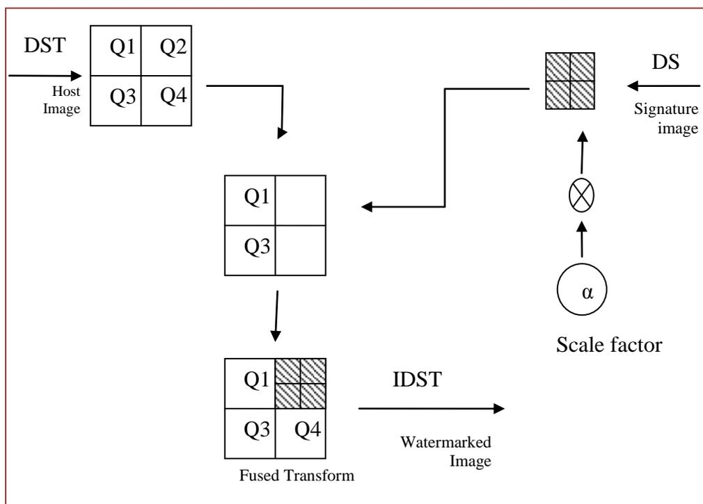
**Fig. (4) A schematic of the data embedding approach**
