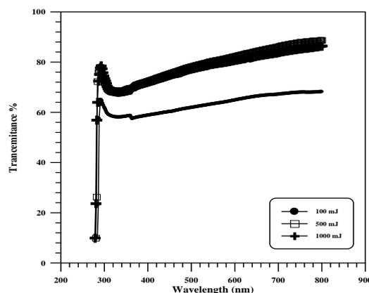
Fig. (1): The transmittance spectra of SnO<sub>2</sub> thin films.
