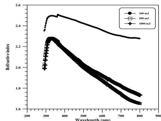
**Fig. (5): The variation of refractive index as a function of wavelength for  $\text{SnO}_2$  thin films**
