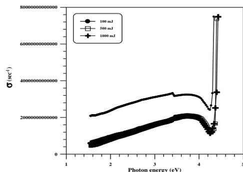
**Fig. (6): The variation of optical conductivity as a function of photon energy for SnO<sub>2</sub> thin films**
