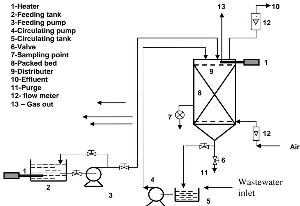
Fig. (1): Schematic diagram of the packed bed system.
