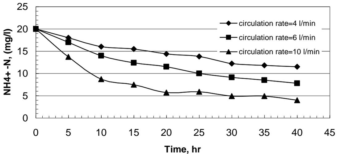
Fig(5) : Effect of circulation rate on Nitrate concentration. (Inoculums conc. =3% T=37°C, packing is Polypropylene mesh, 20 mesh.)
