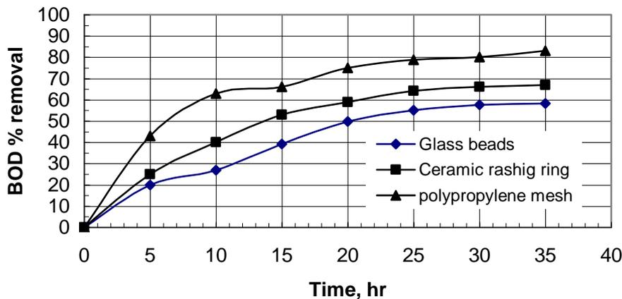
Fig(7): Effect of packing type on BOD removal. (Inoculums conc. =3% , circulation rate = 10 L /min., T=37 °C.)
