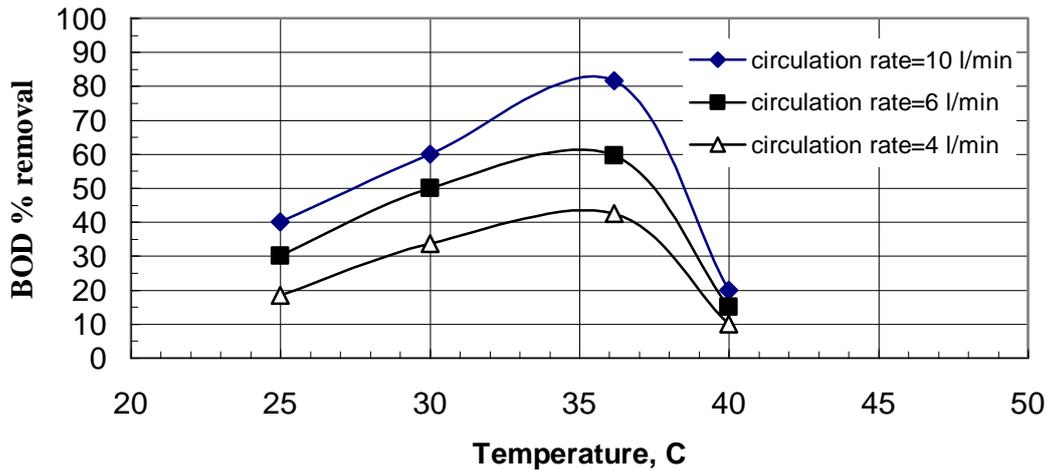
Fig.(6); Effect Temperature on BOD removal. (Time =35 hr, Inoculums conc. =3% , Circulation rate = 10 L /min., packing is Polypropylene mesh, 20 mesh.).
