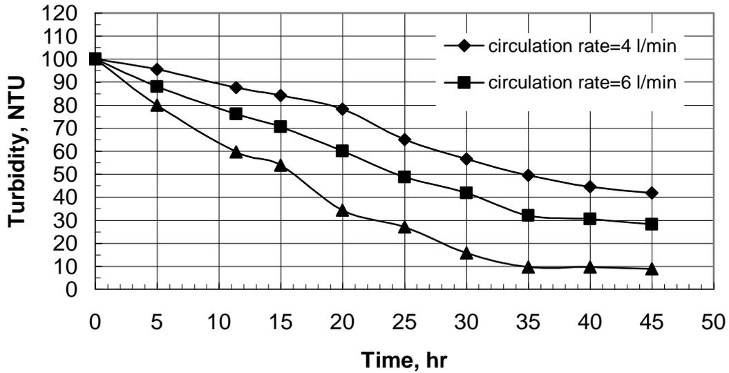
Fig. (4): Effect of circulation rate on turbidity of wastewater. (Inoculums conc. =3% T=37°C, packing is Polypropylene mesh, 20 mesh.)
