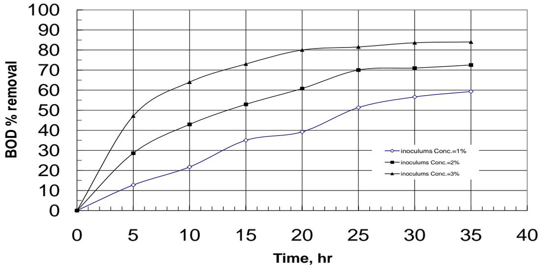
Fig. (2); Effect of inoculum concentration on BOD removal. (Circulation rate =10 L/min., T=37°C ,packing is Polypropylene mesh, 20 mesh.)
