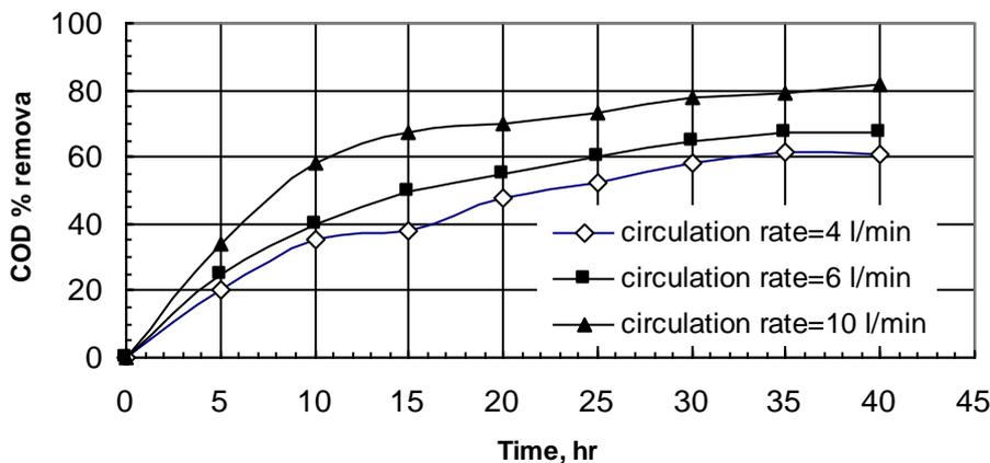
Fig.(3): Effect of circulation rate on COD removal. (Inoculum conc. =3%, T=37°C, Packing is Polypropylene mesh, 20 mesh.)
