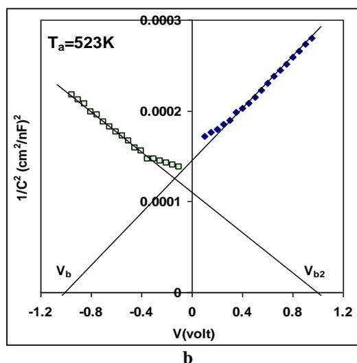
Fig. (5) Built-in voltage of the as-deposited  $\text{In}_2\text{O}_3$  -Si heterojunction, and annealed at 523K
