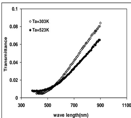
Fig. (3) Transmittance spectrum of the as-deposited  $In_2O_3$  thin films, and annealed at 523K
