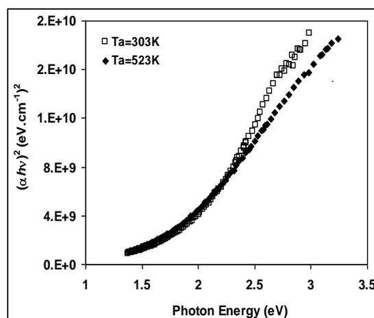
Fig. (4)  $\alpha h\nu$  vs.  $h\nu$  for samples as prepared and annealed at 523K
