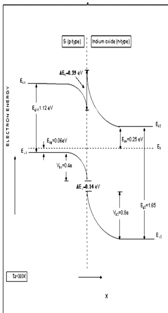
Fig. (6) Energy Band diagram of the as-deposited n- $\text{In}_2\text{O}_3$ /p-Si Heterojunction.
