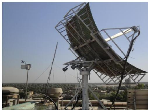
Fig. (4) Photographic of PTSC setup
