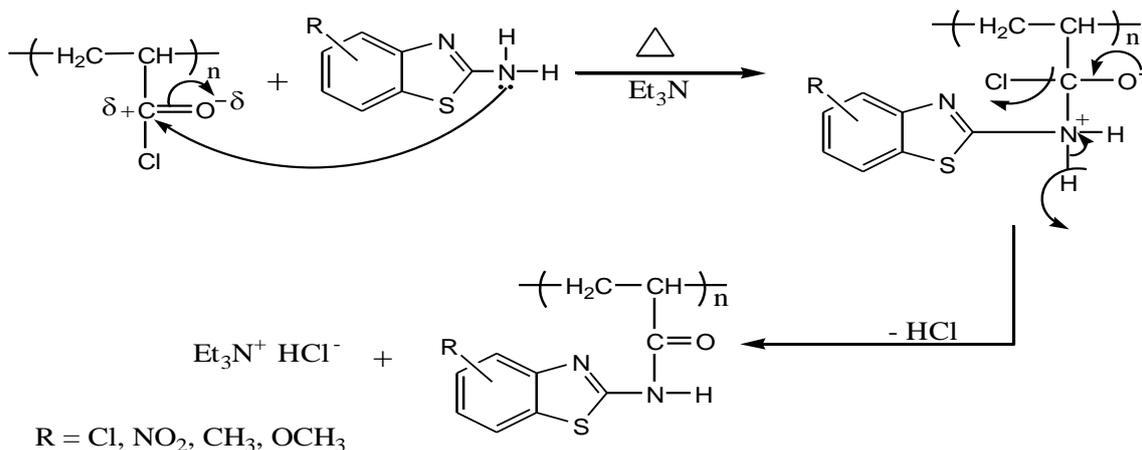
**Scheme (1): Mechanism of preparation of poly [2-(N-acryl)amido substituted benzothiazole]**
