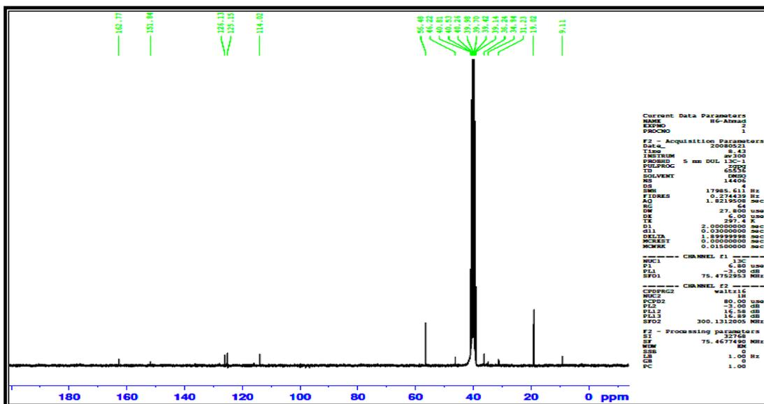
Fig.(9) : <sup>13</sup>C-NMR spectrum of polymer [2]
