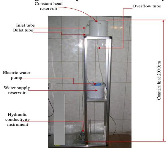
Fig. 6. General View of hydraulic conductivity test rig.
