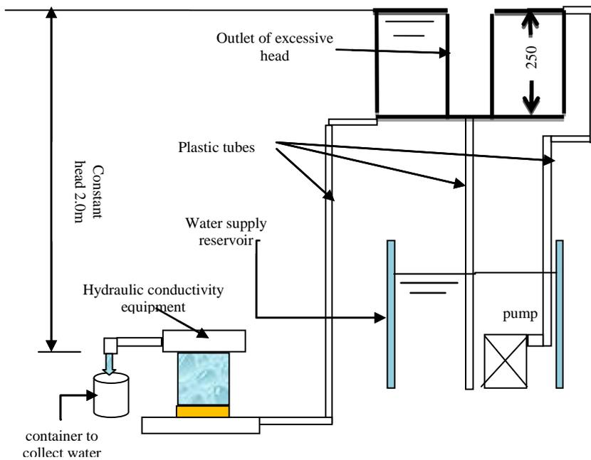
Fig.7. Schematic diagram of hydraulic conductivity test rig.
