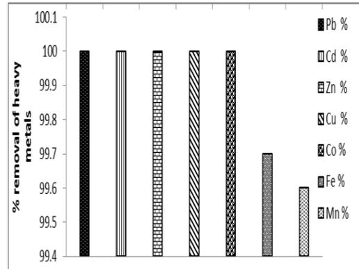
Fig 9: % of removal of heavy metals at concentration 1mg/l.
