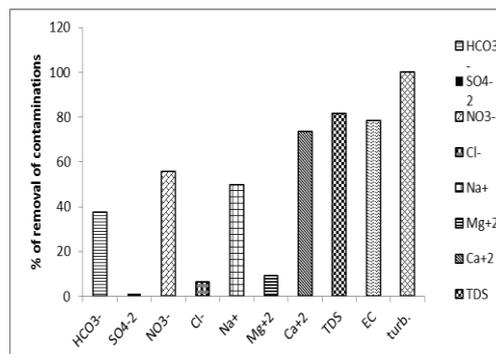
**Fig. 12. % of removal of different contaminations by CP.**
