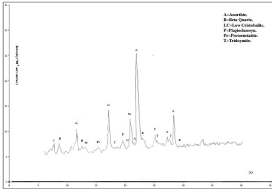
Fig. 8: X-Ray Diagram of ceramic disc filter.
