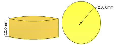
Fig.1– Filter Ceramic Disc Dimensions
