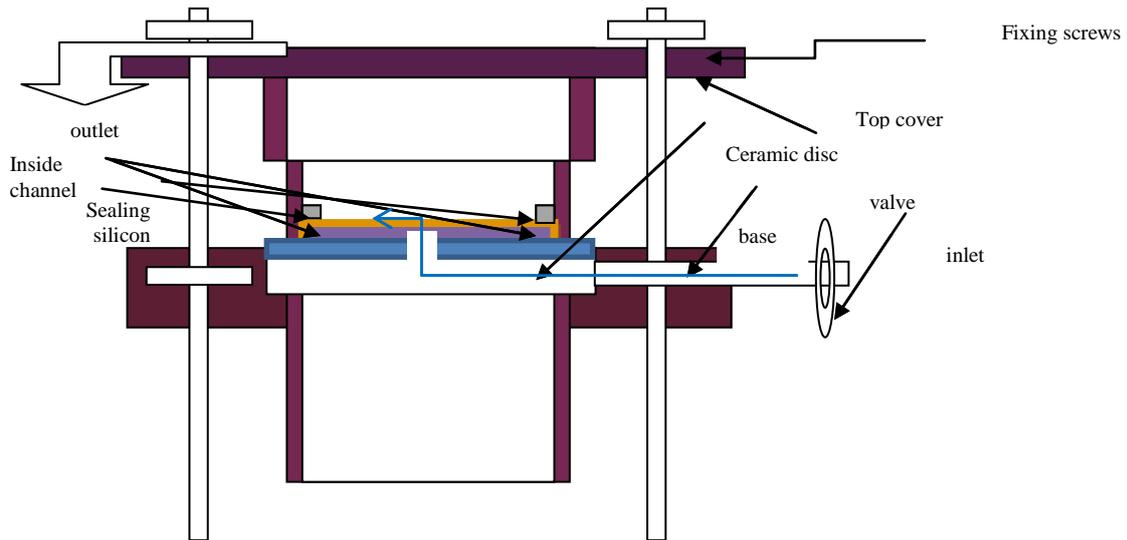
Fig. 5. Schematic diagram of hydraulic conductivity test equipment.
