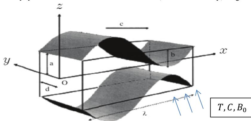
**Figure 1. Schematic diagram for peristaltic flow in a rectangular duct**
