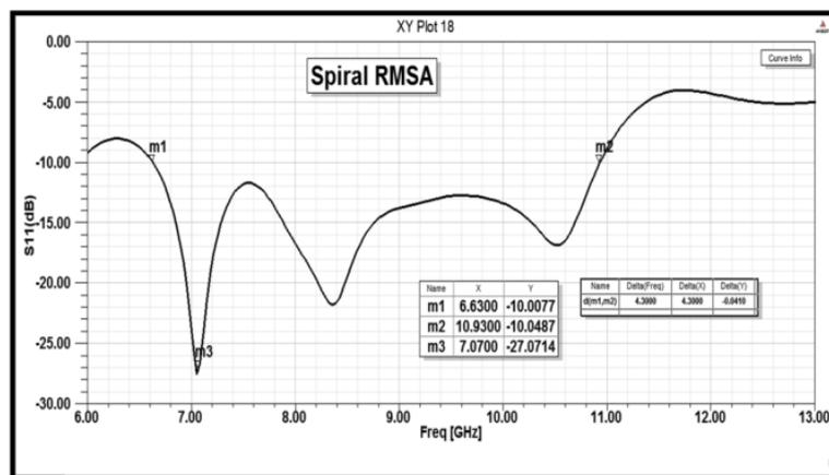
Figure 3. Simulated return loss of proposed antenna.
