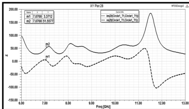
Figure 6. Simulated input impedance of the proposed antenna.
