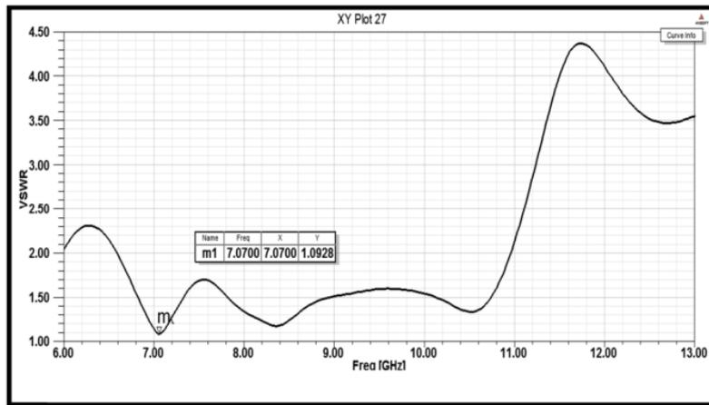
Figure 4. VSWR simulation of the proposed antenna.
