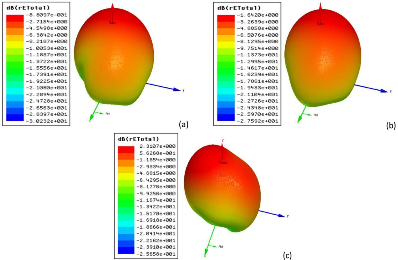
Figure 7. Radiation patterns of designed antenna in 3D: (a)  $f=6.63$  GHz, (b)  $f=7.07$  GHz, and, (c)  $f=10.93$  GHz.
