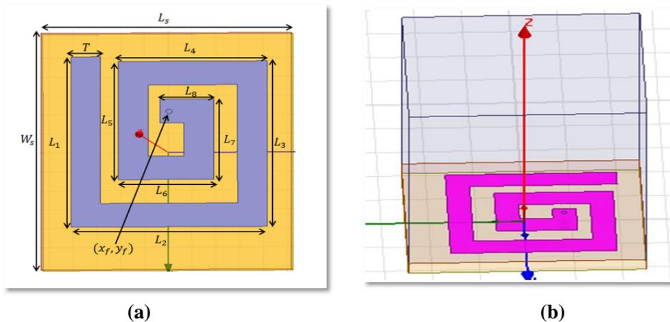
Figure 2. Geometric design and dimensions of the proposed antenna: (a) top view and (b) side view.
