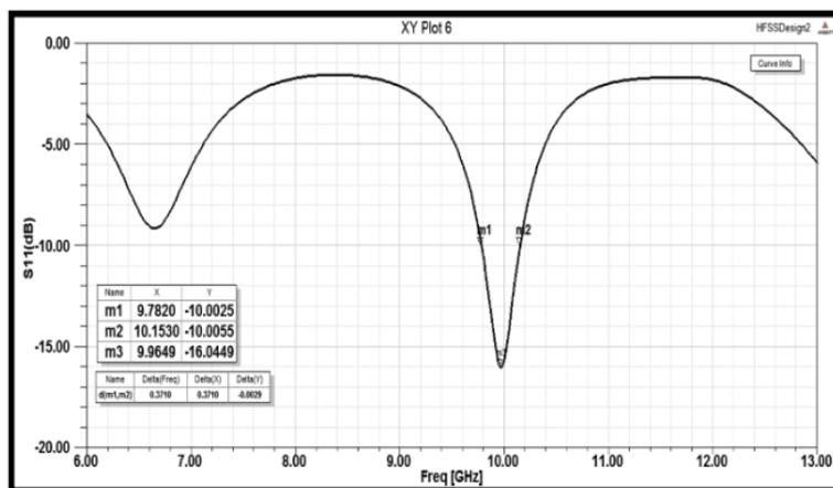
Figure 5. Simulated return loss of RMSA.
