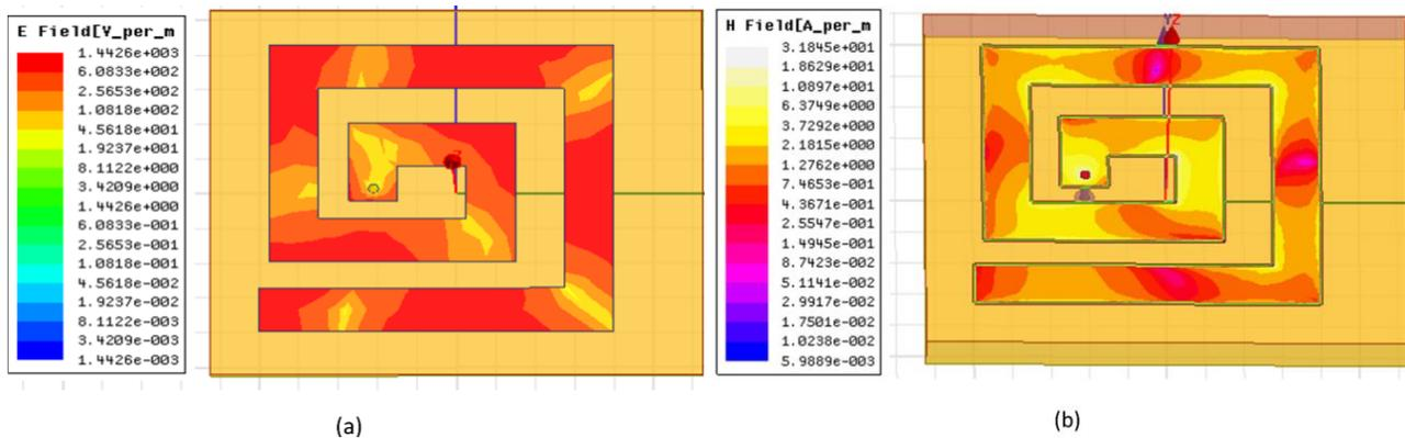
Figure 8. Simulated (a) electric, and (b) magnetic fields distribution on the proposed antenna.
