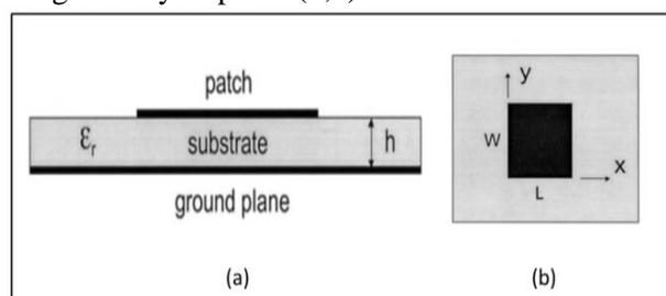
**Figure 1. Geometry of MSA: (a) side view and (b) top view (3).**
