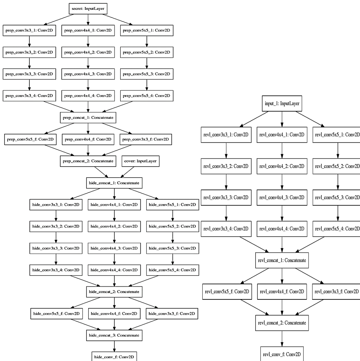
Figure 3. Proposed System Architecture. (a) Hide network, (b) Reveal Network
