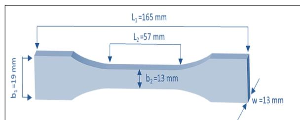
Figure 2. Final ZrO<sub>2</sub> epoxy nanocomposite specimen according to ASTM D638, L<sub>1</sub> = length overall, L<sub>2</sub> = length of narrow section, b<sub>1</sub> = width overall, b<sub>2</sub> = width of narrow section, w = thickness.
