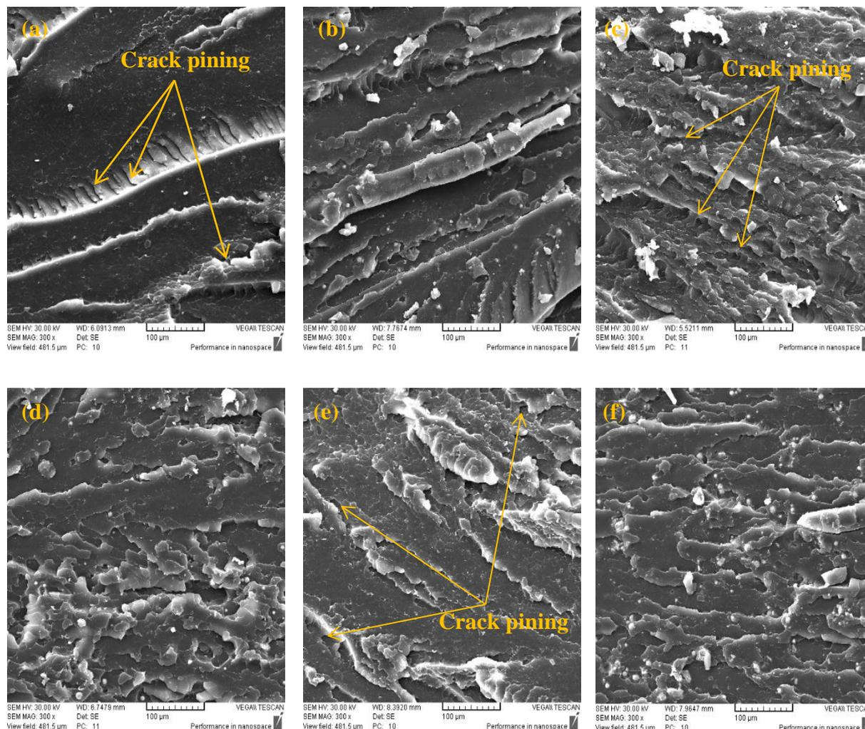
**Figure 8.** SEM images of fracture surfaces of (a) neat epoxy and (b-f) ZrO<sub>2</sub> epoxy nanocomposites of 2%, 4%, 6%, 8%, and 10 vol.% of ZrO<sub>2</sub> nanoparticles respectively, images scale: 100 µm.
