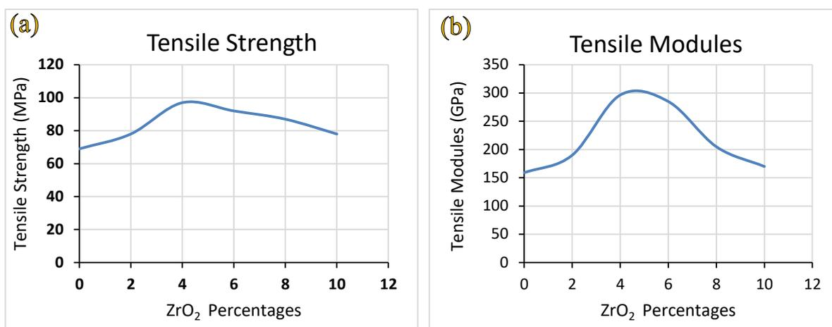
Figure 3. (a) Tensile strength and (b) tensile modules of  $ZrO_2$  epoxy nanocomposites
