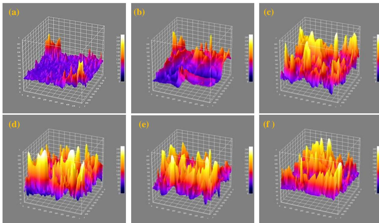
**Figure 7.** 3D heights variation for fractured surfaces of (a) neat epoxy and (b-f) ZrO<sub>2</sub> epoxy nanocomposites 2%, 4%, 6%, 8%, and 10 vol.% of ZrO<sub>2</sub> nanoparticles respectively.
