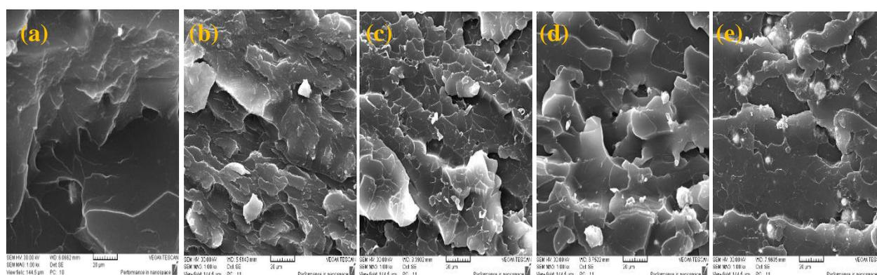
Figure 5. SEM images of fracture surfaces of (a-e)  $ZrO_2$  epoxy nanocomposites of 2%, 4%, 6%, 8%, and 10 vol.% of  $ZrO_2$  nanoparticles respectively and 20  $\mu m$  scale.
