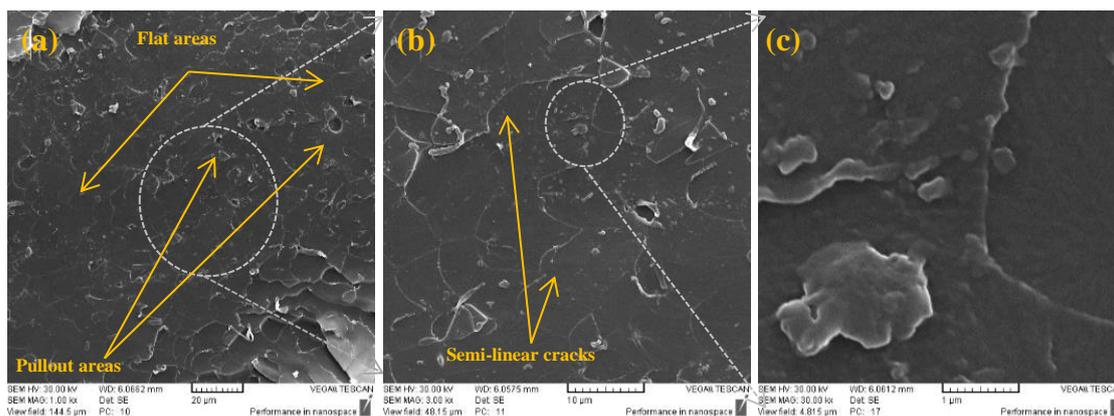
Figure 4. SEM images of the fracture surface of neat epoxy (a) 20  $\mu\text{m}$  (b) 10  $\mu\text{m}$  (c) 1  $\mu\text{m}$  scales
