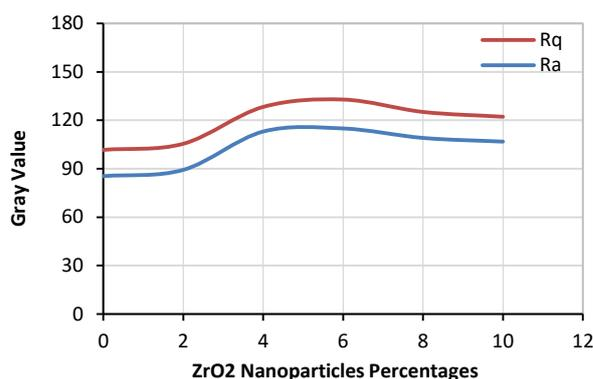
Figure 6. shows the main roughness (Ra) and RMS roughness (Rq) of the fractured surfaces of epoxy nanocomposites and neat epoxy.
