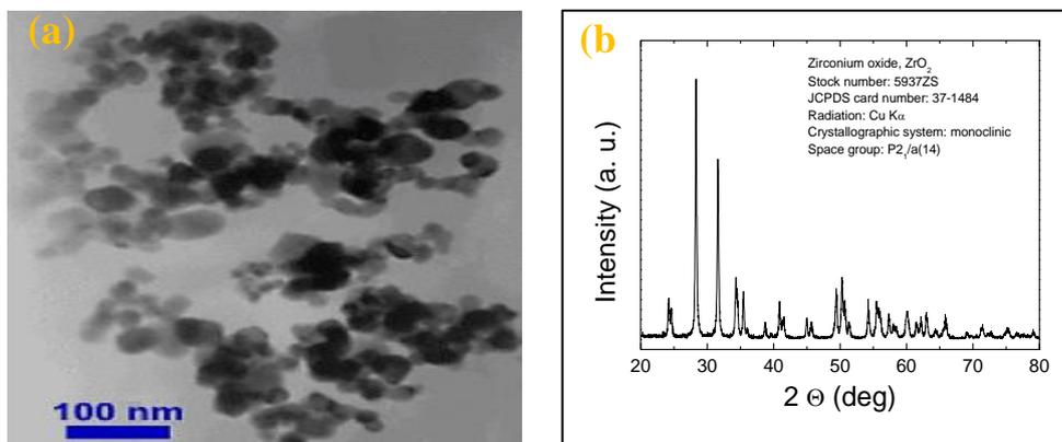
Figure 1. (a) TEM image and (b) X-ray for of ZrO<sub>2</sub> nanoparticles (both supply by MTI company)
