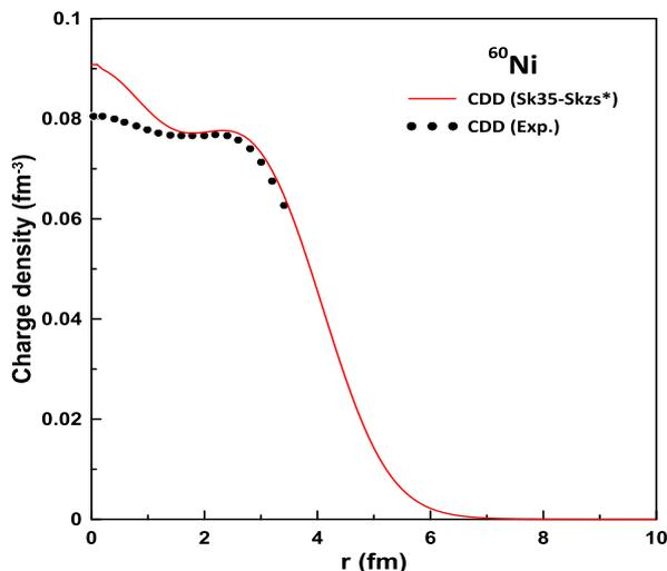
Figure 4. Charge density distribution for  $^{60}\text{Ni}$  using Skyrme parameterization "Sk35-Skzs\*". Measured data from<sup>21</sup>.
