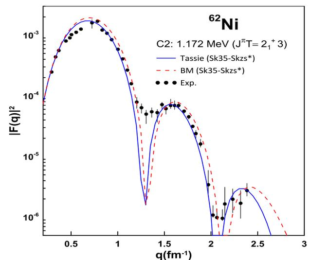
Figure 5. C2 form factor for the  $2_1^+ 3$  state in  $^{62}\text{Ni}$ . Measured data from<sup>22</sup>.
