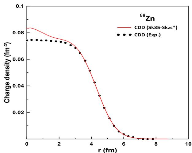
Figure 12. Charge density distribution for  $^{68}\text{Zn}$  using Skyrme parameterization “Sk35-Skzs\*”. Measured data from<sup>23</sup>.
