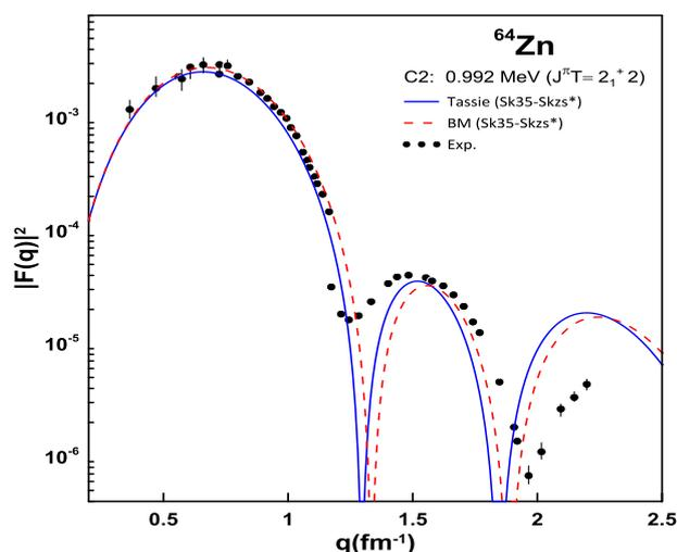
Figure 7. C2 form factor for the  $2_1^+ 2$  state in  $^{64}\text{Zn}$ . Measured data from <sup>23</sup>.
