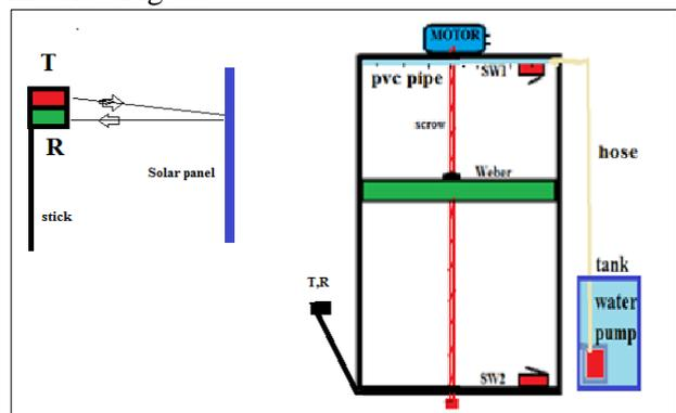
Figure 8. In the right diagram for system components, in the left the instillation package of transmitter, receiver.
