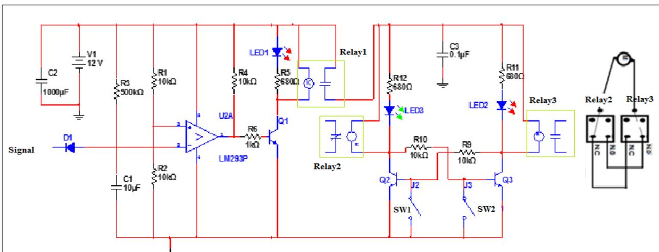
Figure 7. The control circuit to drive water pump and DC Motor .
