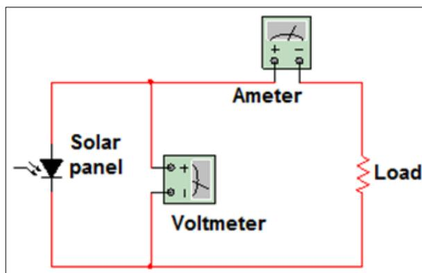
Figure 2. Represents the experimental circuit for testing solar panels.
