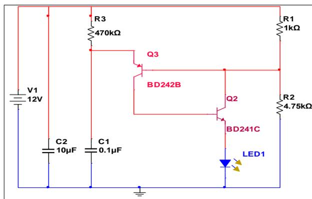
Figure 5. Shows the infrared transmitter.
