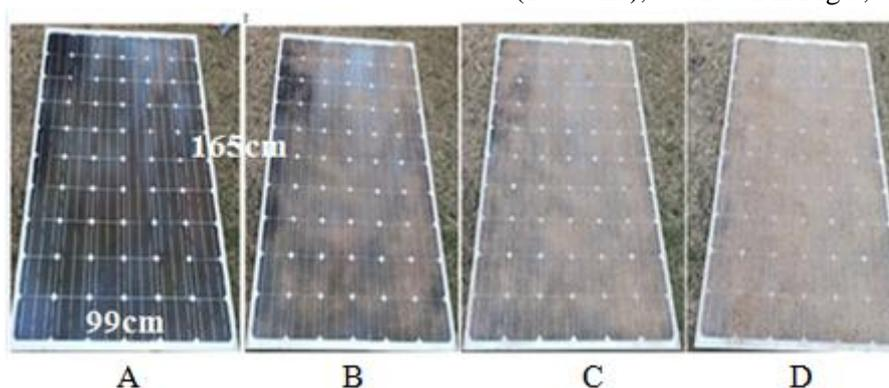
Figure 1. Shows A clean solar panel, B, C, D after adding dust with different weights.
