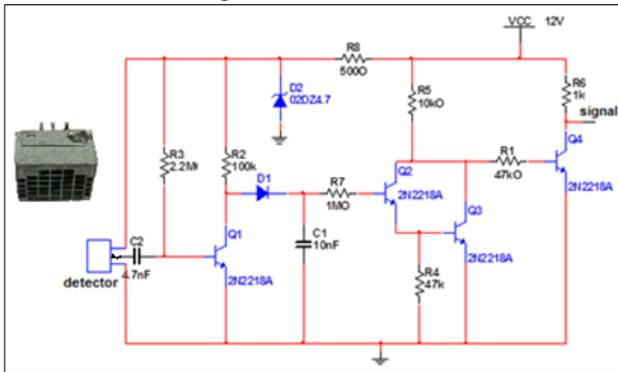
Figure 6. Shows the receiver circuit .
