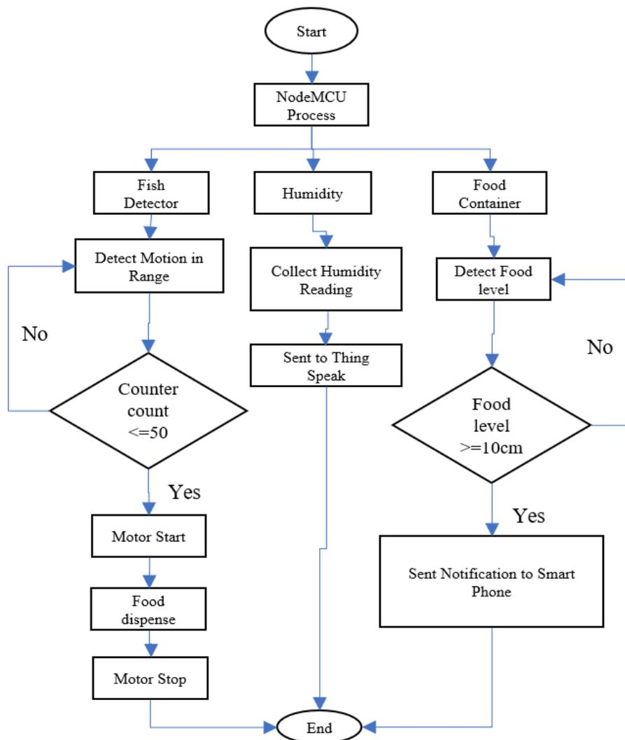
**Figure 1. Flowchart of Automatic Fish Feeder**
