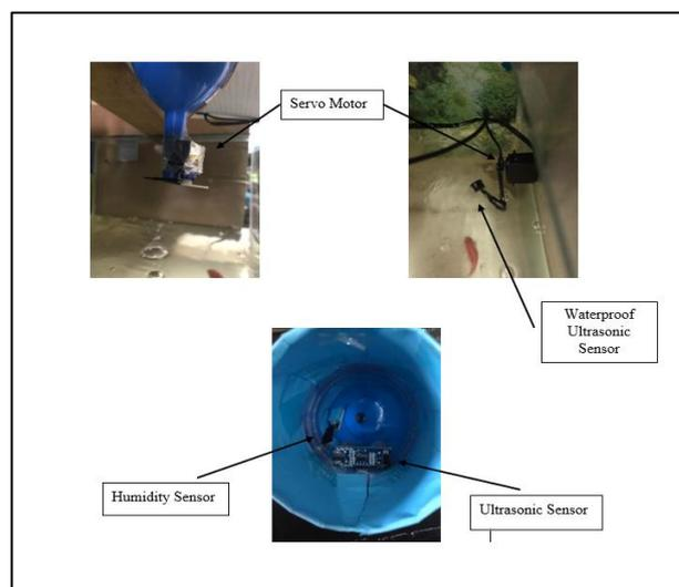
Figure 7. Placing the sensor.
