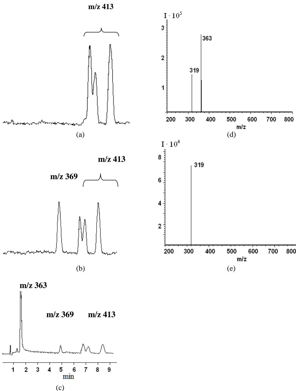
**Figure 3.** Mass chromatograms of ultrafiltrates of the culture fluid of *P. plecoglossicida* DD4 after 0 (a), 24 (b), 72 (c) hours of cultivation in a periodical culture and mass spectra of the MS<sub>1</sub> (d), MS<sub>2</sub> (e) component with m/z 363.
