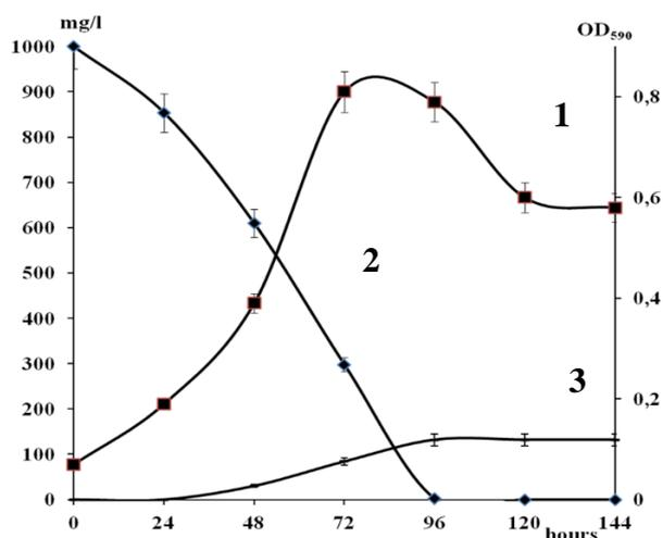
**Figure 2. Dependence of the OD<sub>590</sub> values of the culture fluid (1) and the concentrations of PFOA (2), free fluorine ions (3) in it, depending on the time of cultivation of *P. plecoglossicida* DD4 in a batch culture.**
