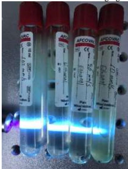
**Figure 11.** The synthesized carbon nanostructure dispersed in ethanol after irradiation with 405 nm laser beam
