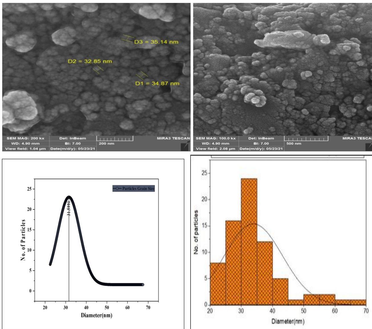
Figure 4. FESEM images of nano binary oxide  $\text{SiO}_2/\text{V}_2\text{O}_5$  and distribution of particle sizes.
