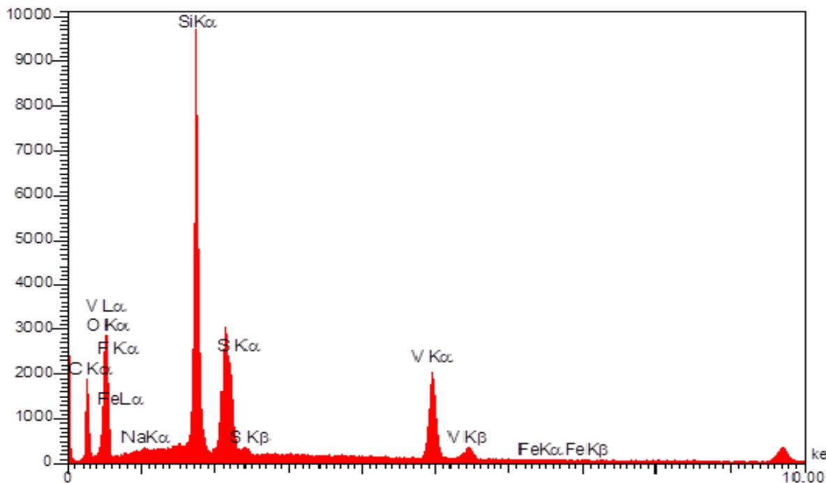
**Figure 3. EDX of nano binary oxide  $\text{SiO}_2/\text{V}_2\text{O}_5$  powder.**
