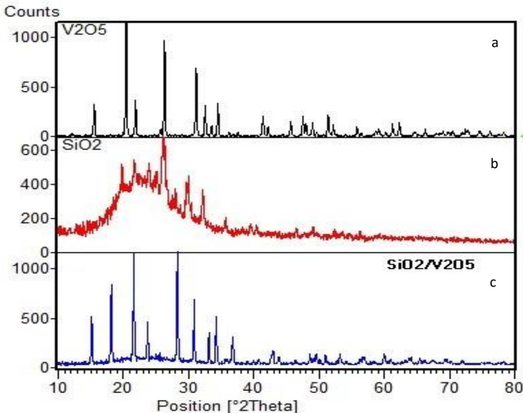
**Figure 2. X-ray diffraction patterns, a. Vanadium pentoxide V<sub>2</sub>O<sub>5</sub>, b. silica oxide and c. nanocomposites SiO<sub>2</sub>/V<sub>2</sub>O<sub>5</sub>.**
