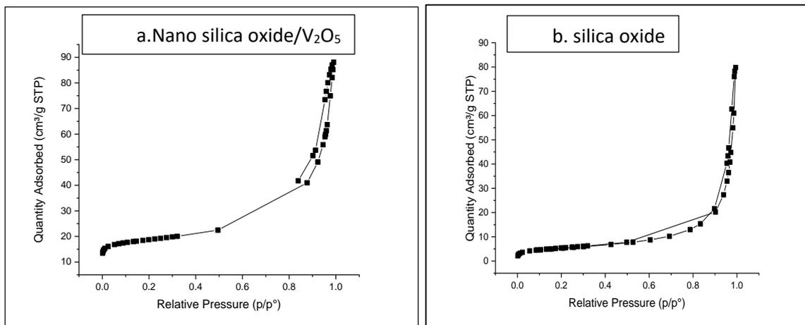
Figure 5. Nitrogen adsorption isotherms for a. nano-silica oxide/ $V_2O_5$  and b. silica oxide.
