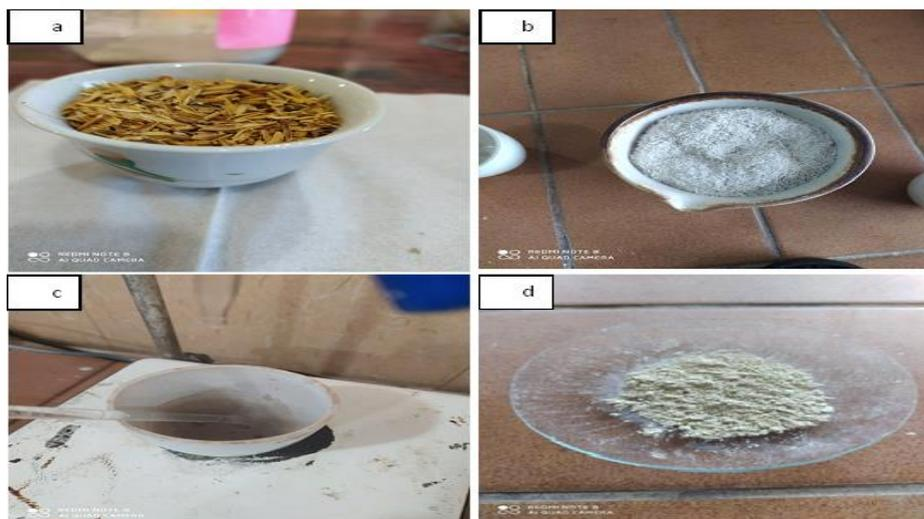
**Figure 1. Preparation steps of silica gel from RHA. A. Rice husk, B. Rice husk ash at 700 °C treatment, C. silica gel, and D. Nano binary oxide SiO<sub>2</sub>/ V<sub>2</sub>O<sub>5</sub> powder.**
