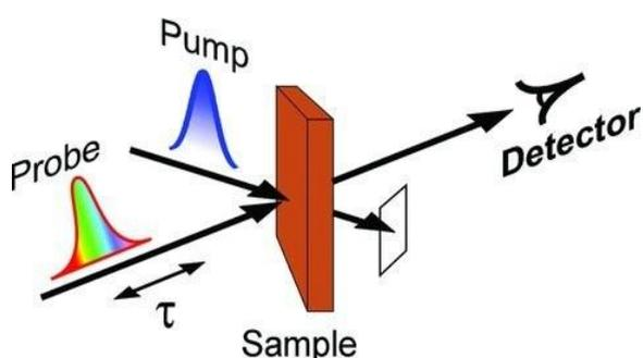
**Figure 1. Scheme of a pump-probe experiment<sup>5</sup>**
