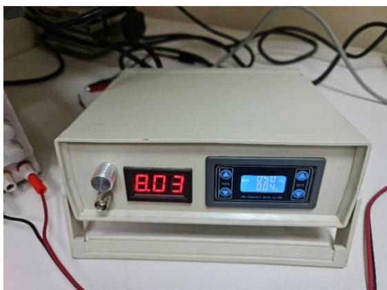
**Figure 4. (PWM) pulse width modulator device**
