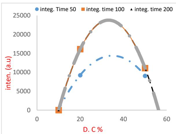
Figure 8. The relation between intensity and pulse width (D.C)
