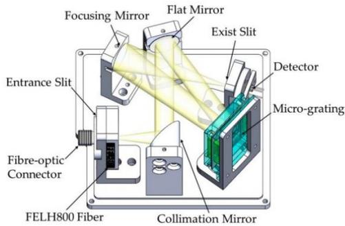
**Figure 5. Drawing of the optical layout and assembly of the spectrometer<sup>14</sup>**
