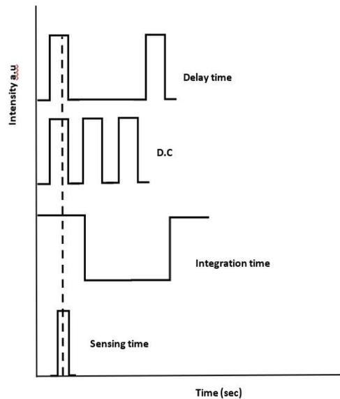
**Figure 6. Operation time sequence of the mean element on the pump-probe system**
