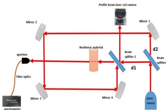
**Figure 4. A scheme for the work of the system that was designed for the (pump-probe) technique**
