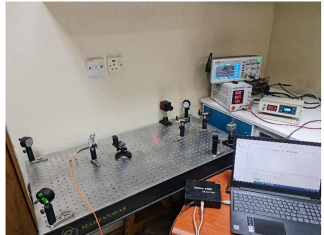
Figure 3. pump probe system
