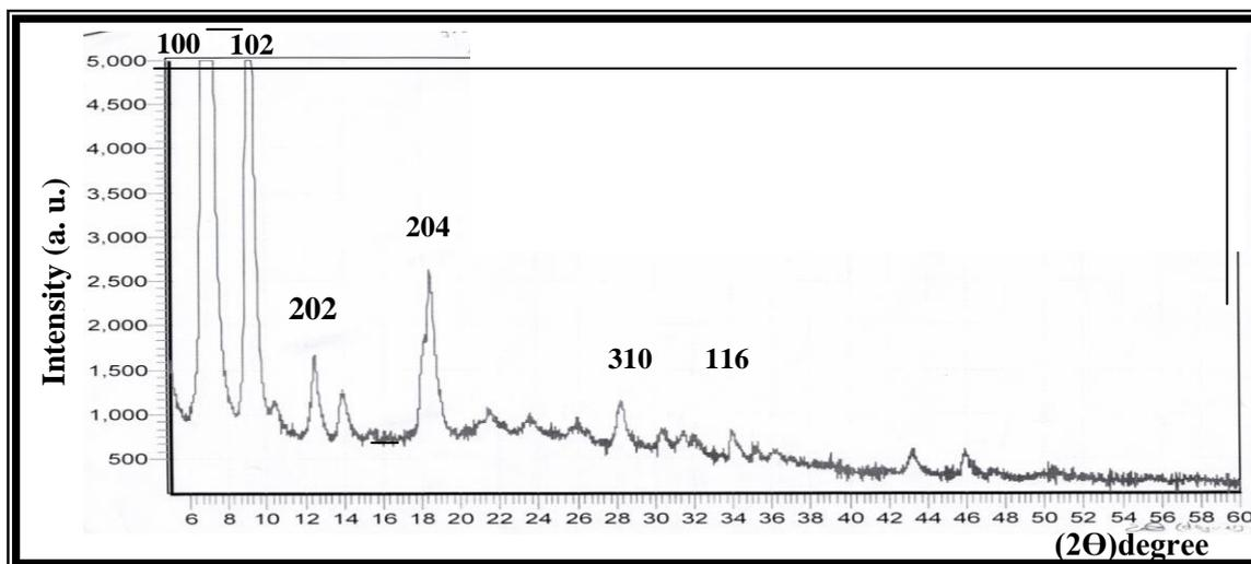
**Fig(3)X-ray diffraction of Zinc-phthalocyanine**
