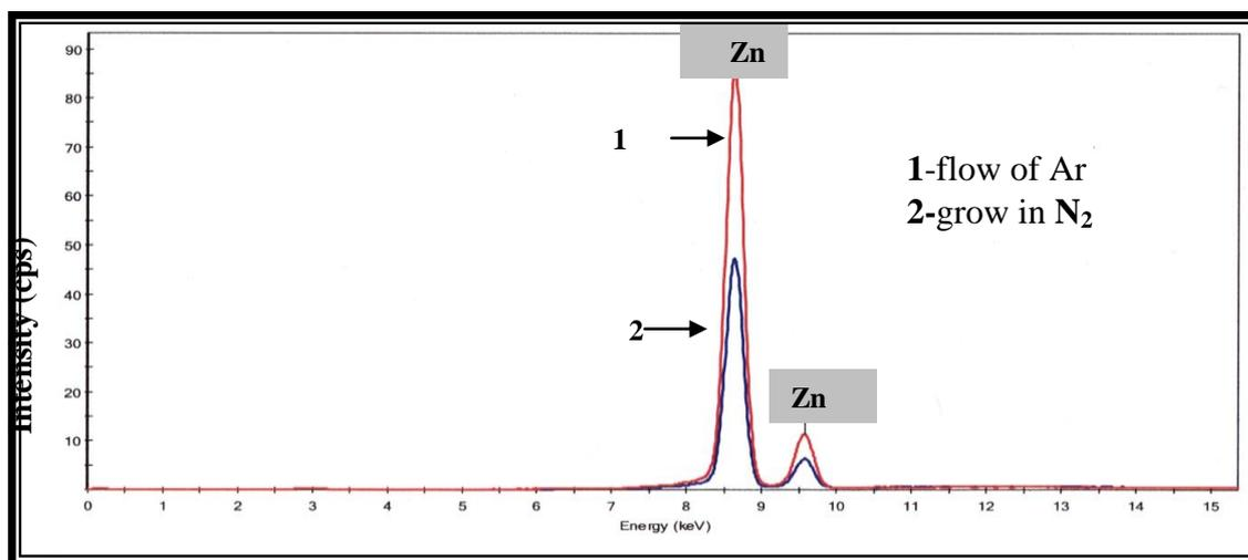
**Fig(2)XRF of zinc phthalocyanine with 1-flow of Ar & 2-grow in N<sub>2</sub>**
