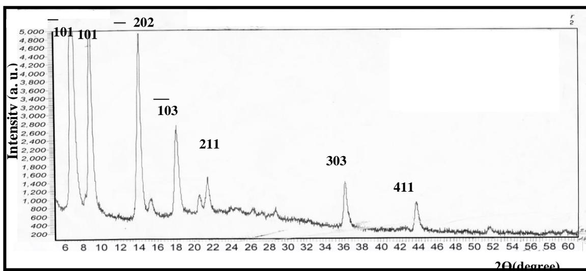
Fig(1)X-ray diffraction of pthalocyanine metal free
