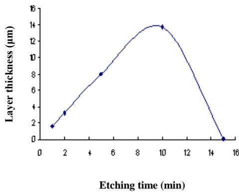
**Fig. (3); The relation between Layer thickness and Etching time.**
