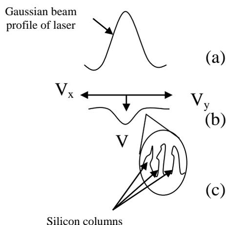
**Fig. (2); A schematic diagram depicts the etching process [8].**
