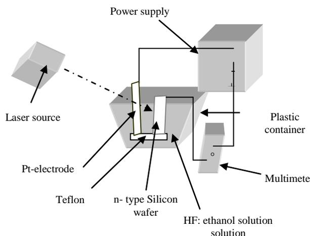
**Fig. (1); Schematic diagram depicts the PEC etching process.**
