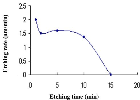
**Fig. (4); The relation between the etching rate and etching time.**
