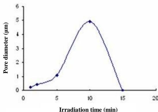
Fig. (9); Effect of etching time on pore diameter.
