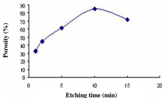
Fig. (8); Effect of etching time on porosity.
