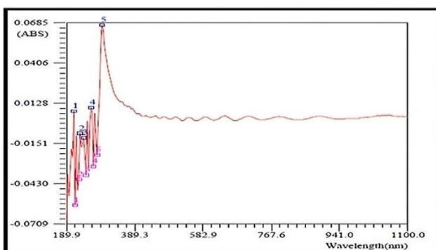
**Figure 5. The absorption spectrum of silver nanoparticles tested by using UV-VIS spectrophotometer.**
