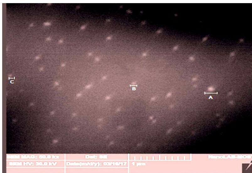
**Image 1.** A scanning electron microscope image showing the shape and size of the nanoparticle prepared with *M. anisopliae* extract; A = 98.2 nm, B = 65.11 nm, C = 35.31 nm.
