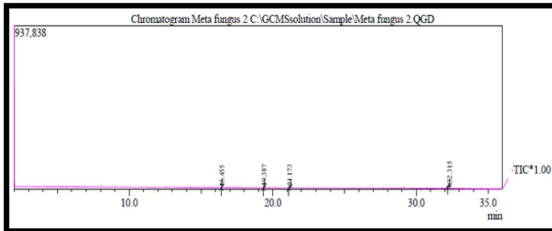
Figure 11. GC-MASS results of a sample of the crude oil treated with silver nanoparticles, showing the decrease in the number and area of the chemical compounds' peaks.
