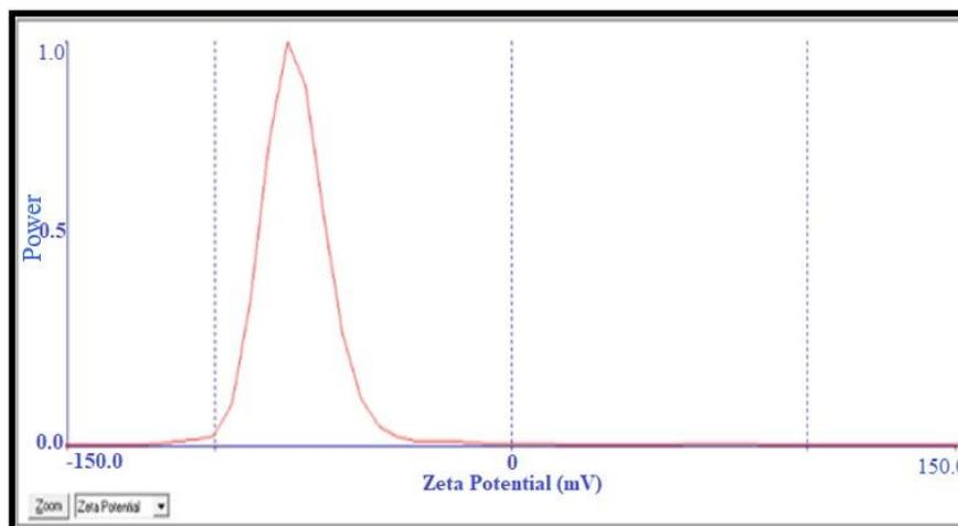
Figure 9. Zeta potential analysis of silver nanoparticles prepared with *M. anisopliae* extract.
