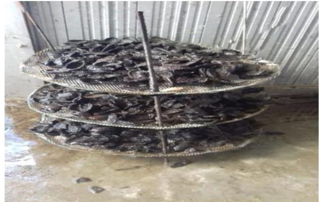
Figure 11. Almond shells are distributed over three layers within the Oxidic tank
