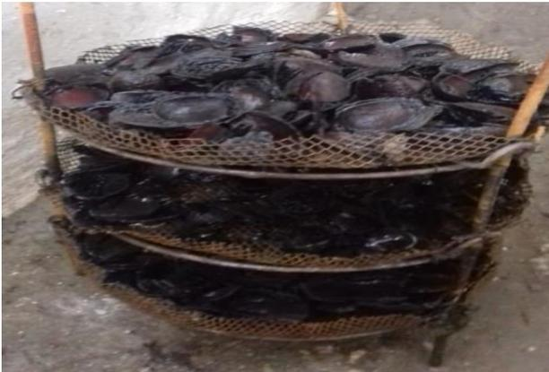
Figure 10. Almond shells distributed over three layers in the Anoxic tank
