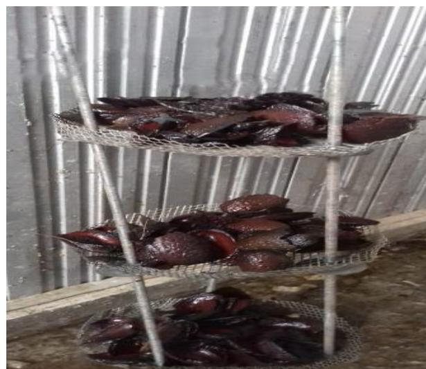
**Figure 9. Almond shells distributed on three layers within the Anaerobic tank**
