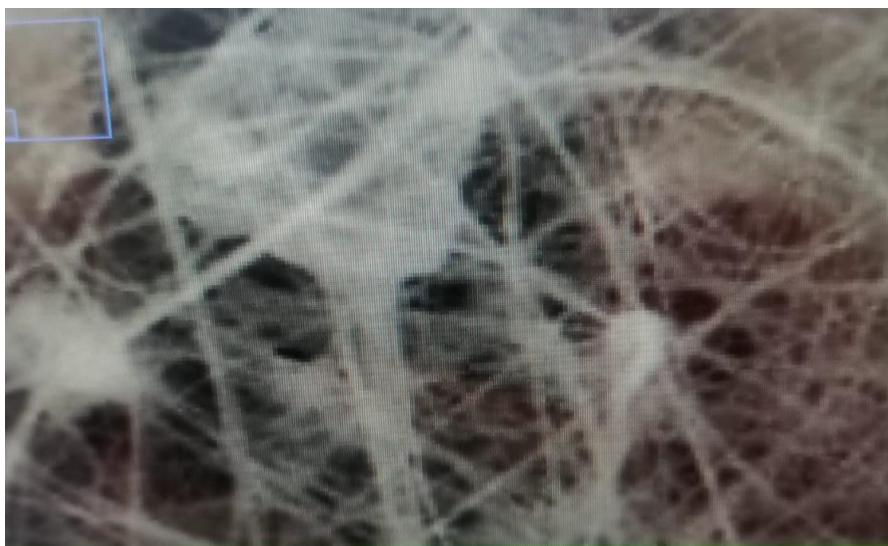
Fig. 15. Using ImageJ software, a magnified image of a bead (at 200% of Fig. 4, 1.25 wt. %) shows an entanglement of fibers.
