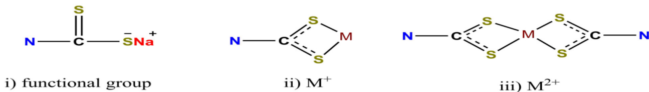
Fig. 1. The dithiocarbamate group attached to heavy metal M. i) functional group, ii) M^+ , iii) M^{2+} .
