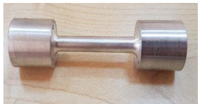
**Figure 2. Tensile specimen**
